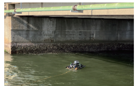
0.1 mm crack detected on a bridge girder's underside even in 10m/s winds using a gimbal camera
