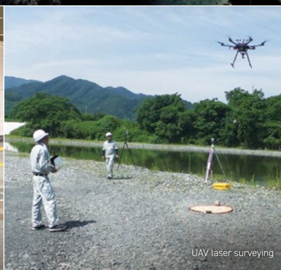
3D topographic data used as basic data for the review of restoration plans for river disasters (Iwate Prefecture)
