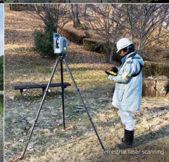
3D topographic data used as basic data for the review of restoration plans for river disasters (Iwate Prefecture)
